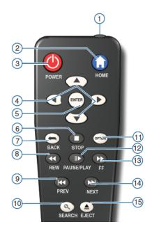
"Option" button is important because it enables OSD messages and menus, in particular - media info, pan & zoom controls, repetition mode (play once, repeat same file, repeat all files in the folder), etc. This button works as on/off toggle switch.
